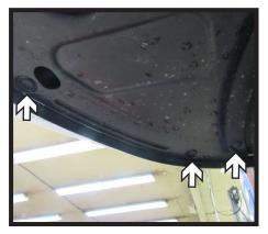
3. Remove the eight (8) push pins from the underside of the fascia.
