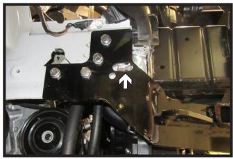
20. On the passenger side of the vehicle remove the front bolt. The bolt will be used when reinstalling the windshield washer fluid reservoir.
