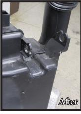
23. **Models w/ Air Baffle**: Remove the two (2) rubber grommets from the air baffle as shown before reinstalling.
