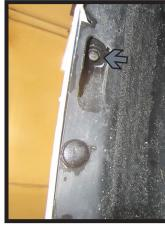
2. Remove the three (3) push pins (white) in front of the tire in the wheel well. Then using a 8MM socket remove the one (1) bolt (gray). Do this on both sides of the vehicle.
