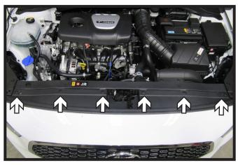
1. Remove the six (6) push pins from the top of the fascia, three (3) on each side.
