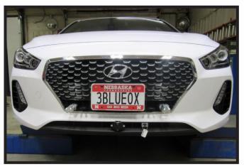
26. Hold the fascia as close to its original position, mark and trim the fascia around the convenience links and attachment tabs. Reinstall the fascia and fascia cover.
