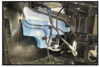
Reinstall the windshield washer fluid reservoir.
