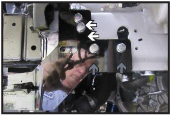
19. Insert two (2) 3/8" bolts (white) into the top two holes with 3/8" whiz nuts and wires on the backside. Insert two (2) 3/8" bolts (gray) into the bottom two holes with 3/8" nut plates and
