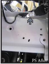
8. Using a 10MM socket remove the two (2) bolts (white) holding wires from both sides of the vehicle frame. On the driver side drill two (2) 1/4" holes as indicated and reinstall bolts (gray). On the passenger side of the vehicle, drill one (1) 1/4" hole as indicated and reinstall both wires using one (1) of the bolts (gray).
