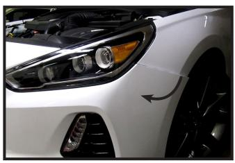
4. To remove the fascia lift and pull the fascia starting by the wheel. Disconnect the running lights as you remove the fascia.
