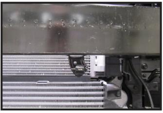
14. Remove the temperature sensor from the bracket. Then using a reciprocating saw remove the temperature sensor bracket from the bumper. The temperature sensor will be relocated later.
