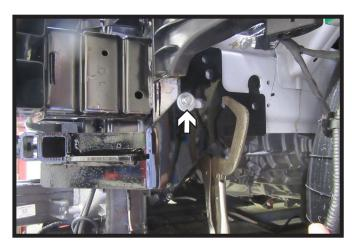
17. Slide the baseplate into position and line up with the existing hole on side of the vehicle. Make sure the baseplate is level. Clamp into place. Insert one (1) 6MM bolt. Do this on both sides of the vehicle.
