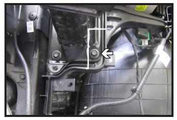
Using a 12MM socket remove the indicated bolt. Then using a reciprocating saw trim the indicated area. Do this on both sides of the vehicle.
