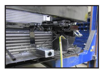
25. Reinstall the temperature sensor to the bottom of the driver side convenience link with included zip tie.
