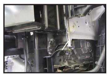
13. Using a reciprocating saw notch a 1" x 1" angled piece from the corner of the indicated area to allow room for the baseplate. Do this on both sides of the vehicle.
