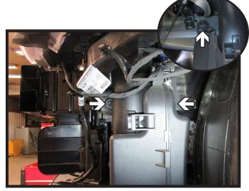
7. **Models w/ Air Baffle**: Using a 10MM socket, remove the three (3) bolts from the air baffle on the driver side of the vehicle. There are two (2) on the outside of the frame and one (1) on the backside. Remove baffle and set aside to be reinstalled later.
