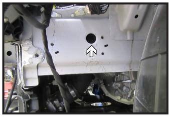
16. Using a 1-1/4" drill bit, drill an access hole as indicated into the side of the frame. Do this on both sides of the vehicle.
