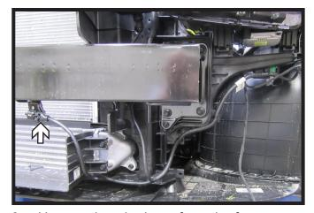
Unsnap the wire loom from the frame.Unplug the temperature sensor (white) and lay down out of the way.
