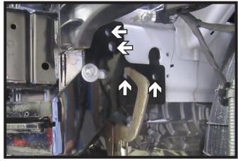
18. Using a 3/8" drill bit, drill the remaining four (4) holes on the baseplate. Do this on both side of the vehicle.
