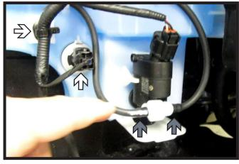
On the passenger side of the vehicle unplug the two (2) wires (white) and two (2) hoses (gray). Mark the hoses first so that they can be reinstalled correctly later.
