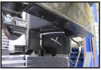
11. Using a utility knife trim the plastic piece as indicated. Do this on both sides of the vehicle.
