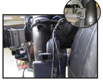
24. **Models w/ Air Baffle**: Reinstall the air baffle on the driver side of the vehicle using the provided 6MM bolt with hardware on the outside of the frame. Use the existing bolt and hardware on the backside of the frame (inset).
