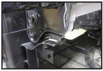
15. Using a utility knife trim the plastic piece as indicated. Do this on both sides of the vehicle.
